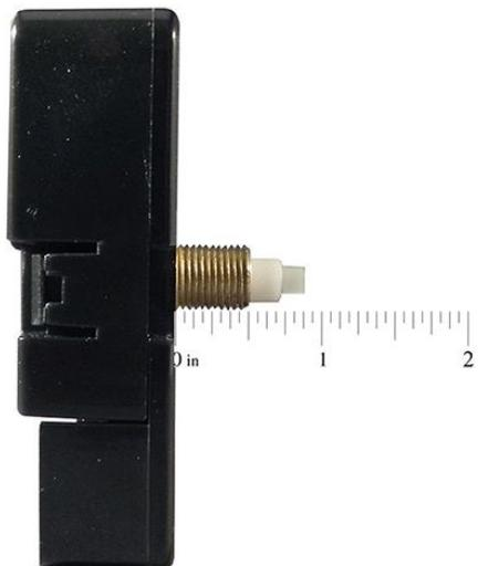
In the case that you simply want to replace a broken motor, there are two measurements you will need from your old motor. The most accurate way to measure the shaft length on a clock motor is to use the depth gauge on a digital caliper. A ruler can be used as well, but make sure the ruler starts at 0, many rulers have their zero point a bit away from the end of the ruler.
